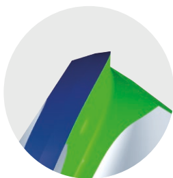
CAD representation of cutting edge and chip space geometry
